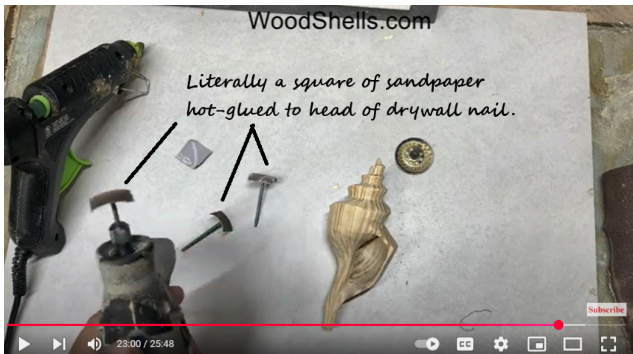
Figure 5. Square sanders are simply a piece of cloth-backed abrasive hot-glued onto the head of a nail for a shank. Works great!
