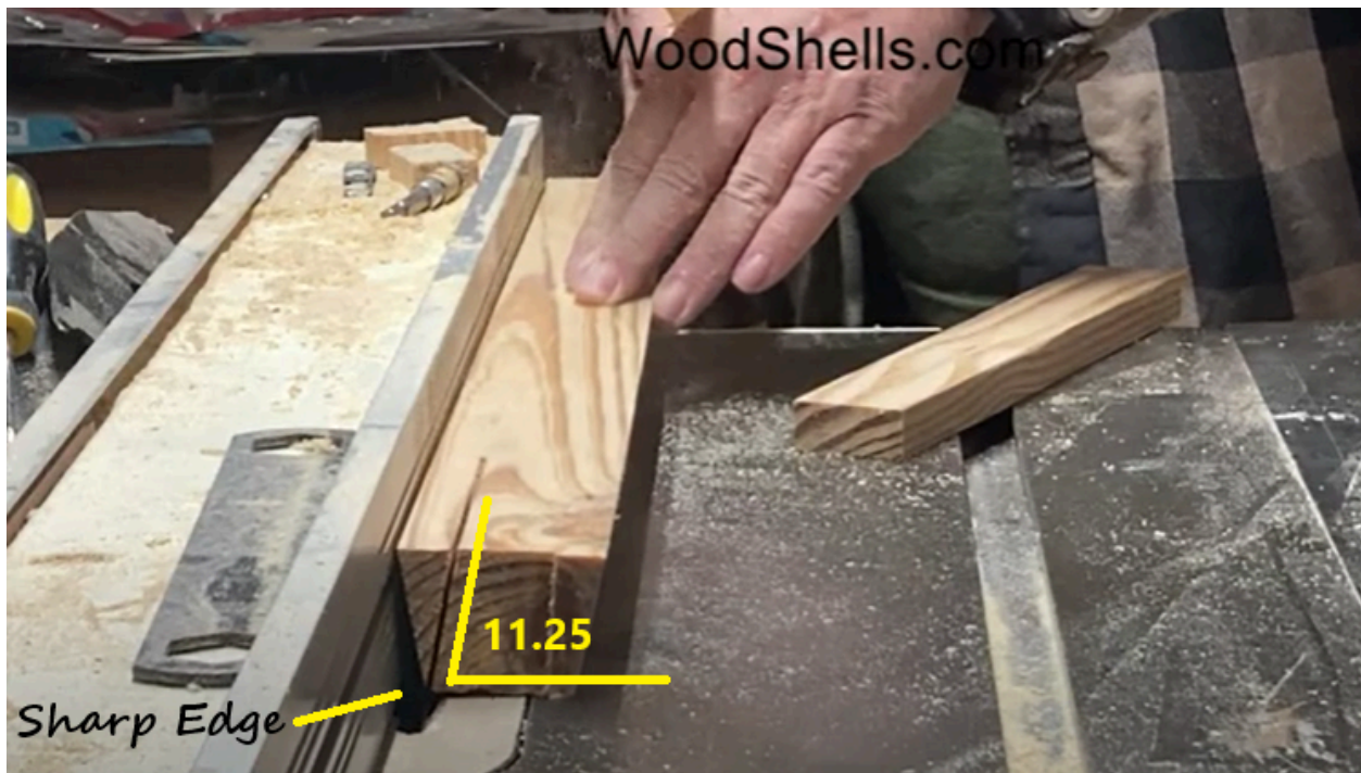
Figure 1. Sawing wedge material on a table saw. After each cut the board is flipped end-over-end to cut the next wedge.
